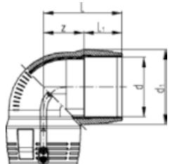
SDR potrubí (SDR 11-17/17,6) – Voda PN 16, plyn PN 10
