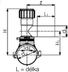
SDR potrubí (SDR 11 - 26) – Voda PN 16, plyn PN 10
